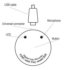
Figure 1: Edic-mini Tiny model B30
