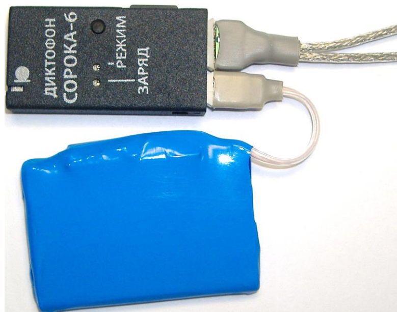
Fig. 7. Example of the voice recorder "SOROKA- 06E" operation with an external accumulator and external stereo microphones.
