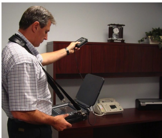
Figure 2 Operator with OSCOR Green portable spectrum analyzer locating IR transmitter
