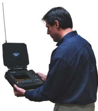
Figure 1 Operator with OSCOR Green portable spectrum analyzer is locating radio source
