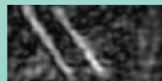
Two reinforcement rods in concrete (depth is 11 cm, distance between rods is 8 cm, frequency is 6.6 GHz)
