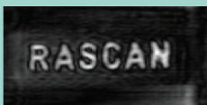
Word "RASCAN" cut from aluminum foil, under 6 cm of foamed concrete (frequency is 6.6 GHz)
